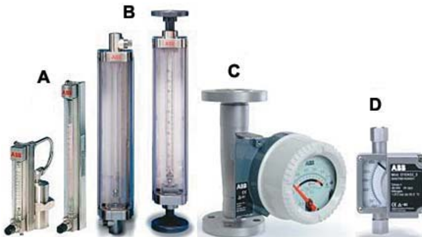
Typical rotameter types widely used in the process industries include two low-capacity meters often used as purge meters (A). (Note the optional scale lengths); higher capacity, "standard" meters (B), shown here with female threaded connections (left) and screw-on pipe flanges (right); metal tube or armored rotameters for higher flow capacities (C) and for low flows including purging (D).
